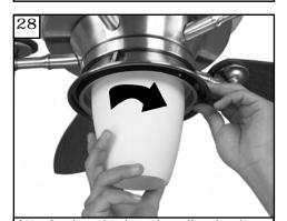
Attach glass by locating dimples in light kit with the groves in glass and twisting clockwise till tight.
